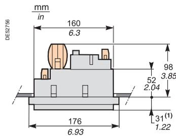
Sepam with basic UMI and MES114, mounted with AMT840 plate.
