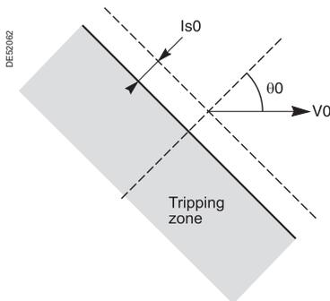
Tripping characteristic of ANSI 67N/67NC type 1 protection (characteristic angle  $q0 = 0^\circ$ ).
