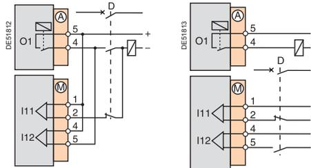
Connection for shunt trip coil monitoring.
