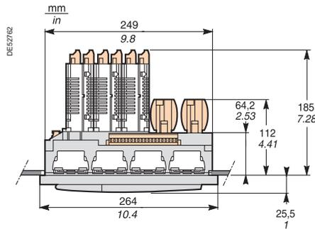
Top view of Sepam with MES120, flush-mounted in front panel with spring clips.
