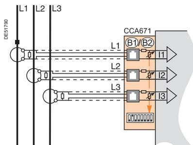
Connection of 3 Low Power Current Transducer (LPCT) type sensors to the CCA671 connector. It is necessary to connect 3 sensors; if only one or two sensors are connected, Sepam goes into fail-safe position.
