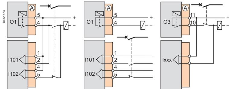
Connection for shunt trip coil monitoring.
