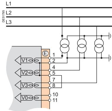
Measurement of the 3 phase-to-neutral voltages allows the calculation of residual voltage,  $V_0\Sigma$ .
