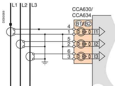
Connection of 3 x 1 A or 5 A sensors to the CCA630 connector.
