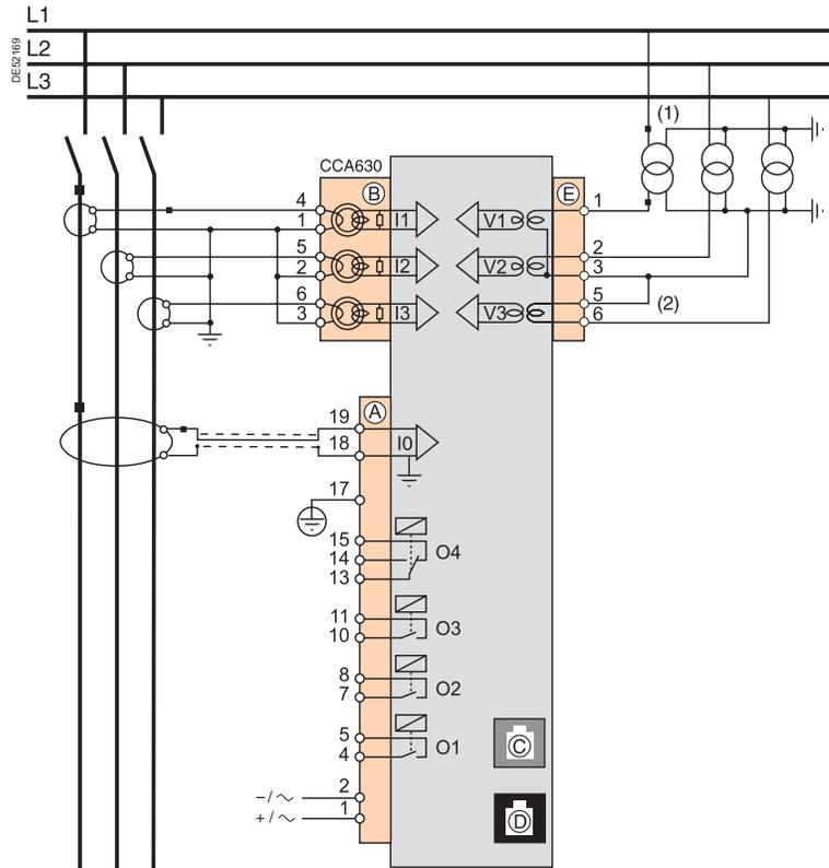
(1) This type of connection allows the calculation of residual voltage.
