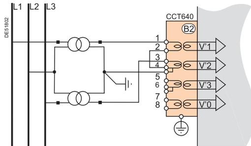
This variant does not allow the calculation of residual voltage.
