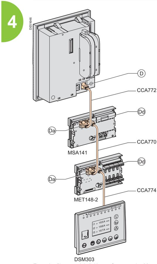
Example of inter-module linking on Sepam series 20.
