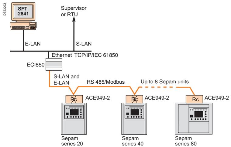
**Note:** Rc = line-impedance matching resistor.
