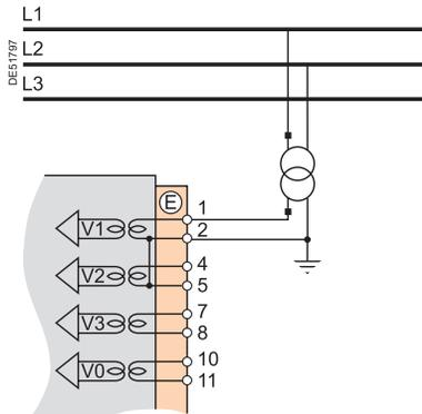
This variant does not allow the calculation of residual voltage.
