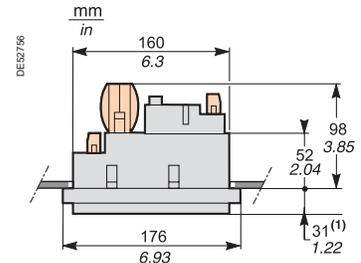
Sepam with advanced UMI and MES114, flush-mounted in front panel.
