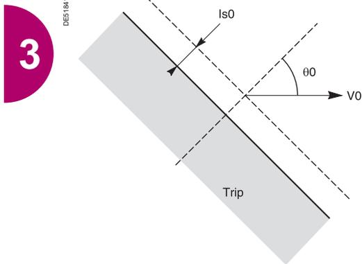
Tripping characteristic of ANSI 67N/67NC type 1 protection (characteristic angle  $\varphi_0 \pm 90^\circ$ ).
