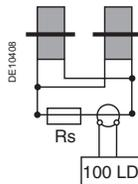
■ **Example 3** (N = 4 blocks per phase): 1 triple module + 1 single module for a single-phase relay.
