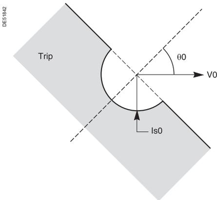
Tripping characteristic of ANSI 67N/67NC type 2 protection (characteristic angle  $\varphi_0 \pm 90^\circ$ ).
