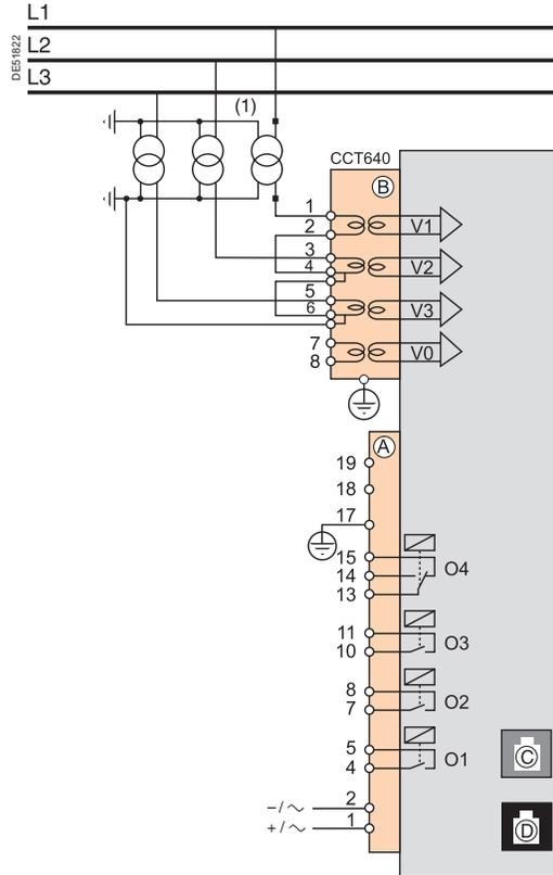
(1) This type of connection allows the calculation of residual voltage.
