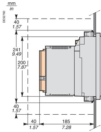
Side view of Sepam with MES120, flush-mounted in front panel with spring clips.
