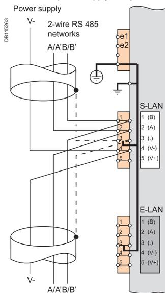
If ACE969TP-2 is used alone, the external power supply is not required, the V- connectors on the modules must be interconnected.
