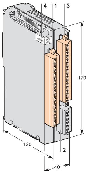
Installation of the second MES120 module, connected to base unit connector H2.
