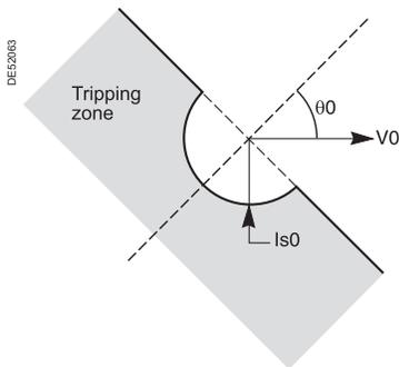
Tripping characteristic of ANSI 67N/67NC type 2 protection (characteristic angle  $q0 = 0^\circ$ ).
