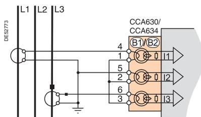
Connection of 2 x 1 A or 5 A sensors to the CCA630 connector.
